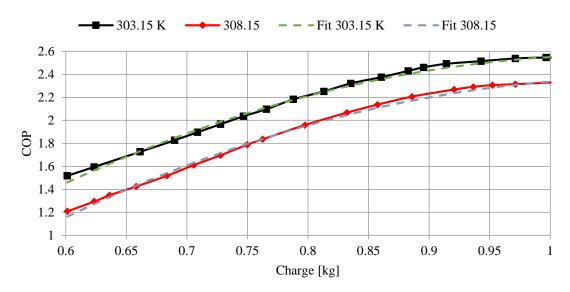
Figure 1: Comparison of experimental and correlated charge degradation data at different indoor temperatures
