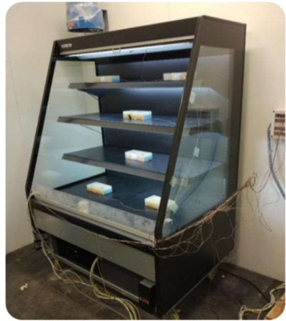
Fig. 1. View of the vertical open-fronted cabinet.
