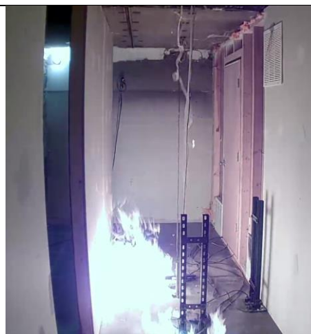
Flames 20s after refrigerant release.
