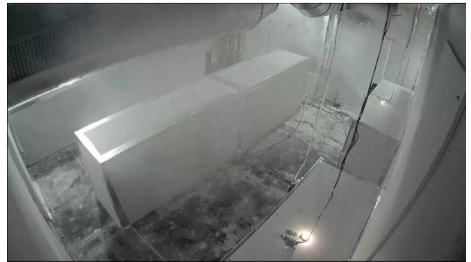
Mist exiting the supply duct at 62 seconds after the beginning of the discharge. The blower motor had been started 2 seconds prior to this frame. Candles at locations C and D extinguished 17 seconds later. The candles at locations A and B remained lit throughout the test.
