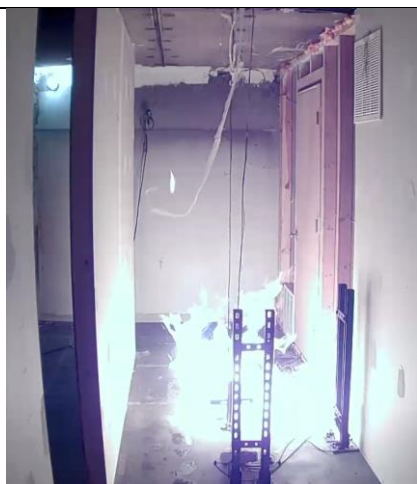
16s after refrigerant release; flame spread observed on the floor in the hallway toward the right wall.
