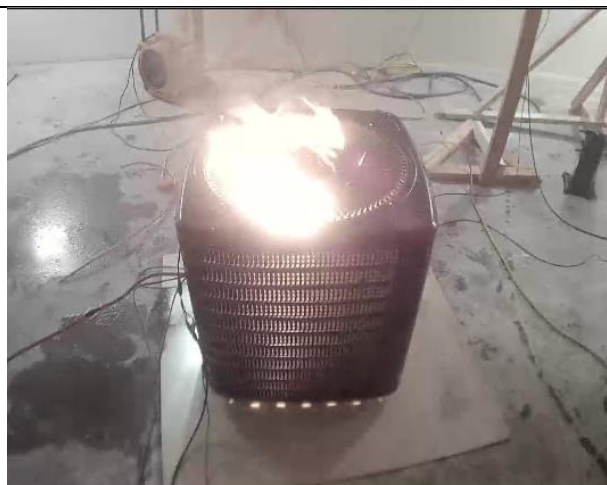
Video still showing ignition (55 s after release start)
