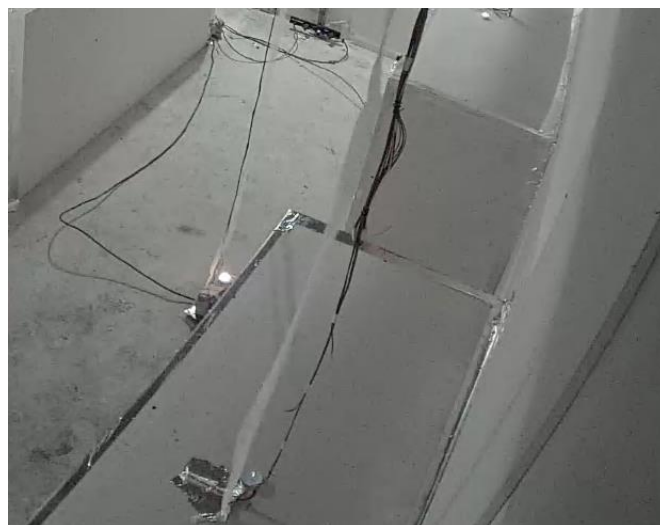
Candles at Locations A, C, D extinguished at 35 seconds after blower motor up to speed (26 Hz).
