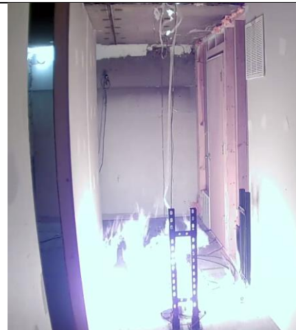
Flames 18s after refrigerant release; flames moves toward the return air grill.
