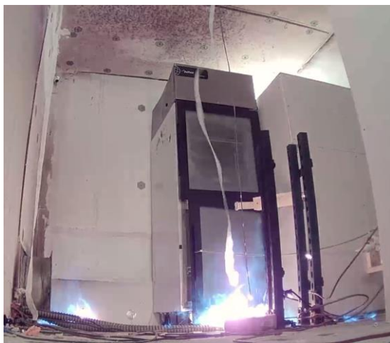
Ignition of refrigerant 6 seconds after the reach-in cooler door was opened showing flaming in front and in corner.
