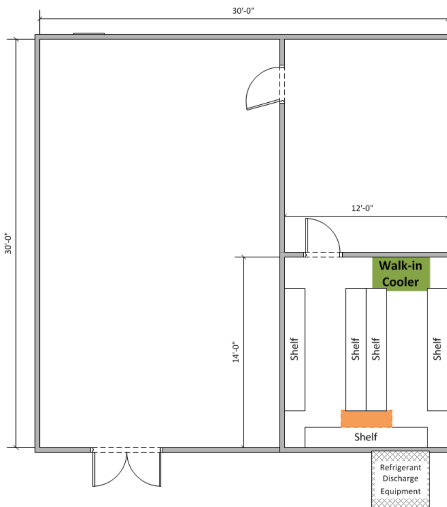
Figure 124 – Walk-in cooler Layout within the 30'x30' test room
