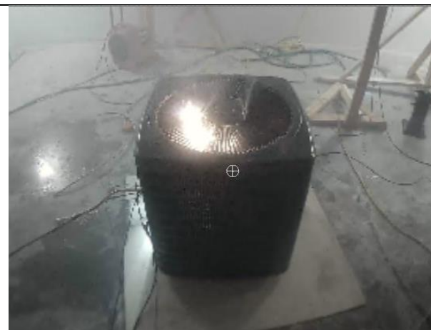
Video still showing ignition (102 s after release start)
