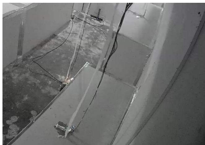
Candles flickering at 34 seconds after the beginning of the discharge. The blower motor had been started 2 seconds prior.
