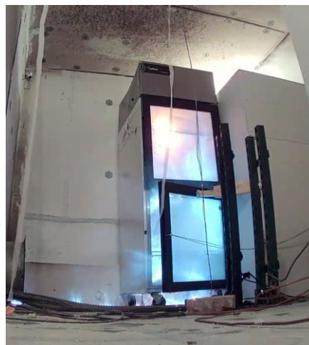
Flames 10s after reach-in cooler door is opened enter the cooler
