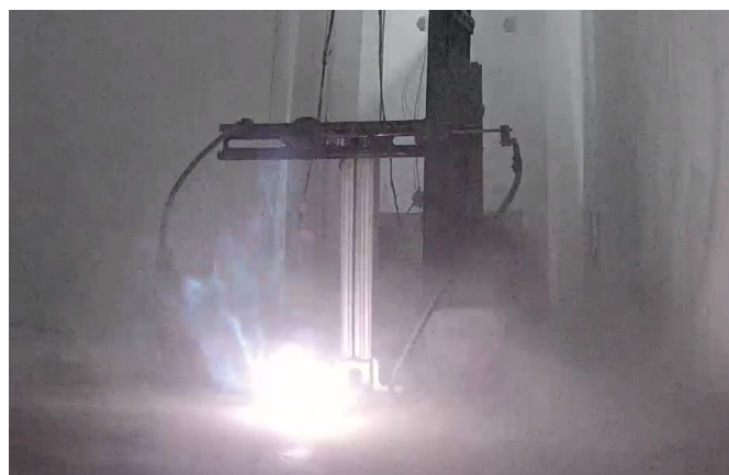
Ignition at floor level 56 seconds after the start of the discharge.
