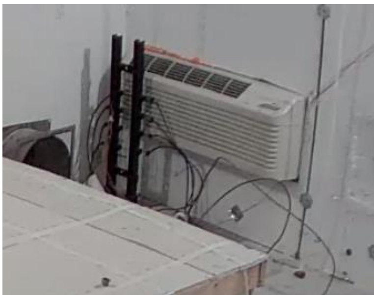
Figure 90 – PTAC installation in test MPTAC01. The PTAC is positioned 3 inches away from the side wall.
