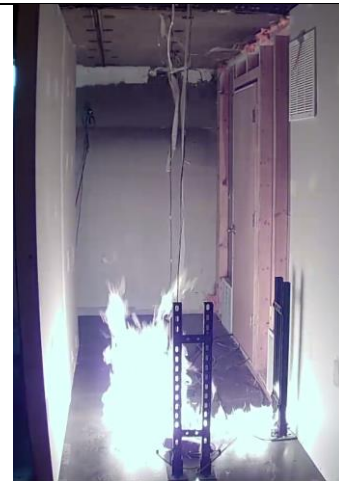
Flames 20s after refrigerant release.
