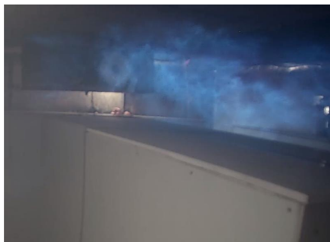
One second after the start of sustained ignition, the flames reached the ceiling of the walk-in. The total duration of sustained flaming was 9 seconds.
