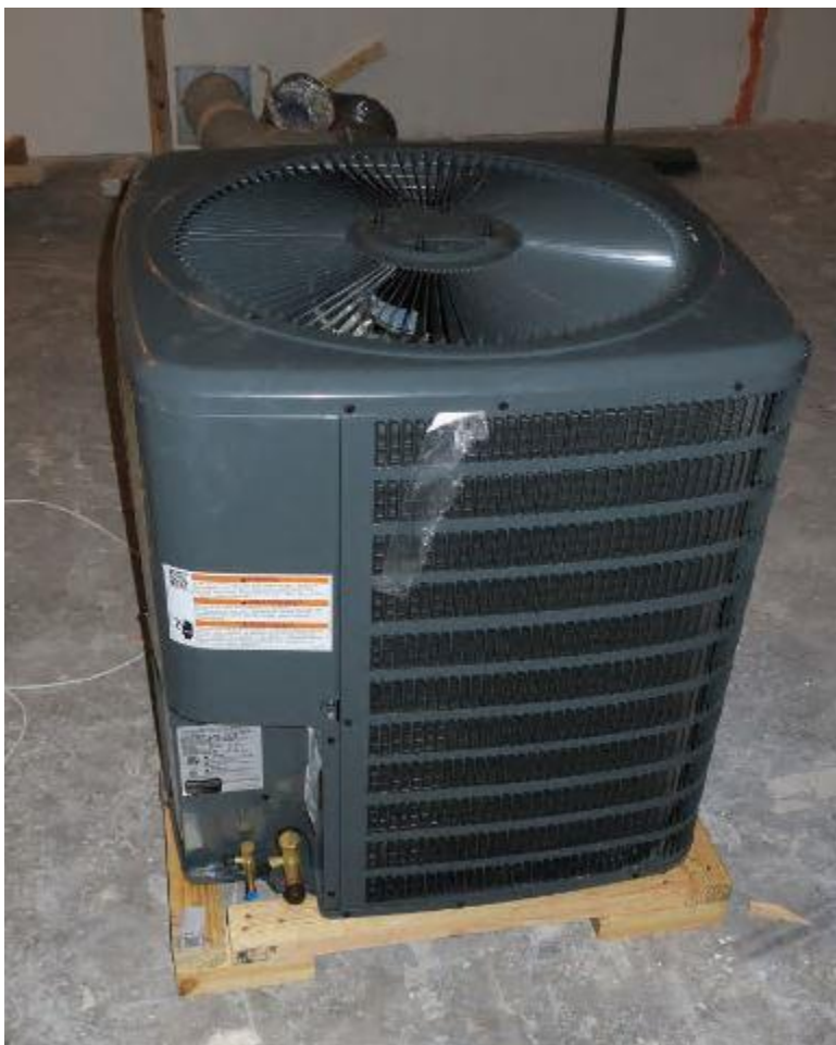
Figure 170 – Outdoor Condenser and Compressor (Hermetic Electrical Pass-Through Terminal Failure Tests)
