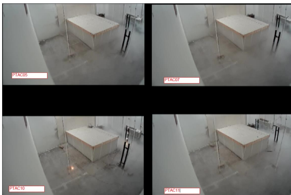
Figure 93 – Comparison of R-452B videos at 35 seconds after the start of release
