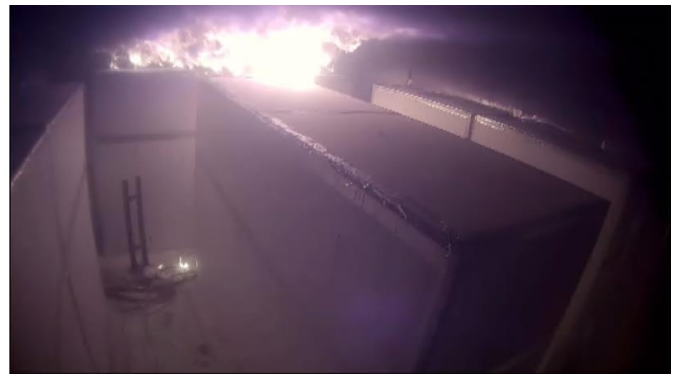
Ceiling level view of flames at ceiling height 93 seconds after that start of the discharge. The ceiling is obscured by smoke.
