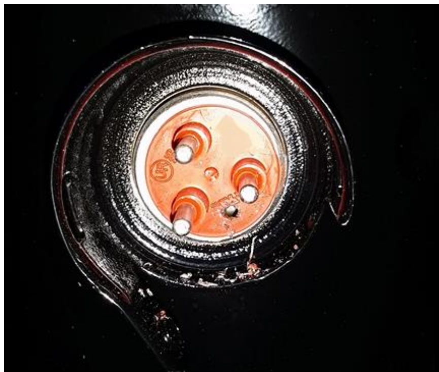
Figure 149 – Location of the intentional hole drilled in the body of the Hermetic Electrical Pass-Through Terminal
