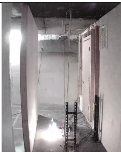
Ignition of the refrigerant 12s after refrigerant release.
