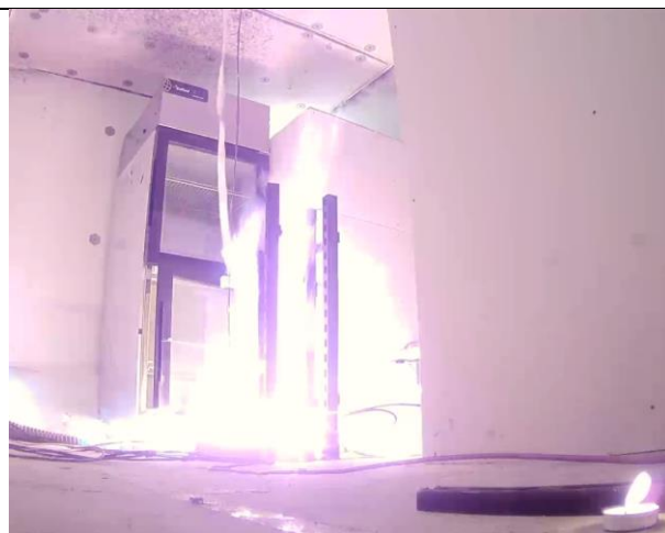
Flames 4s after reach-in cooler door - the fire size grew rapidly.
