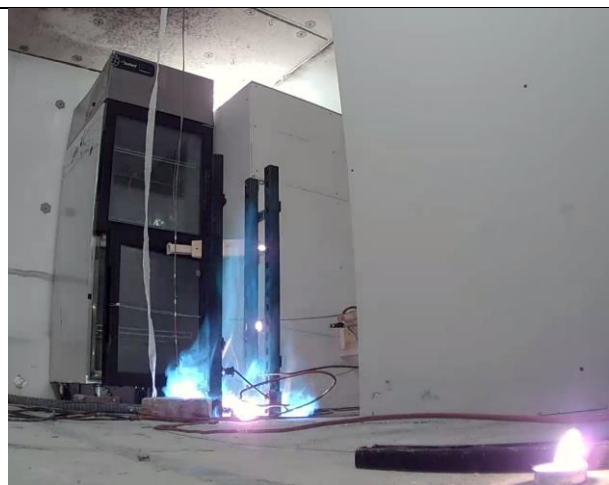
Flames 3 seconds after the reach-in cooler door was opened.
