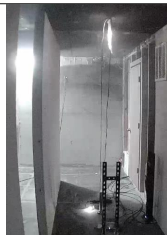
76s after refrigerant release; cheese cloth ignition all the way to the ceiling; all flaming ceased 84s after refrigerant release.
