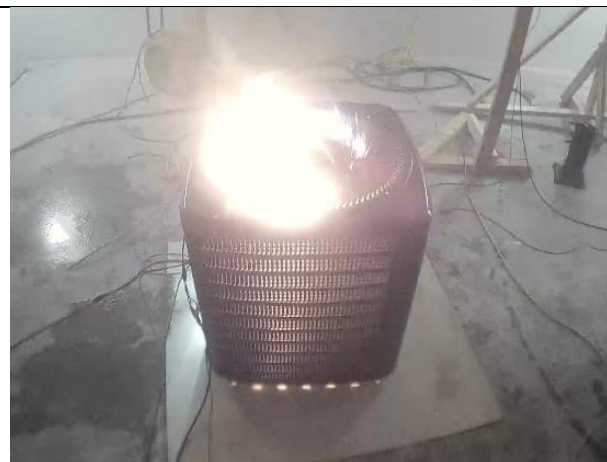
Video still showing ignition (82 s after release start)
