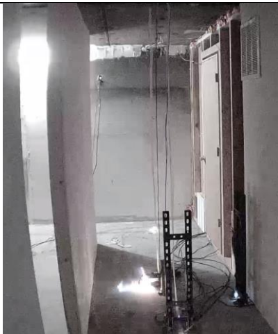
Ignition of the refrigerant 12s after refrigerant release.
