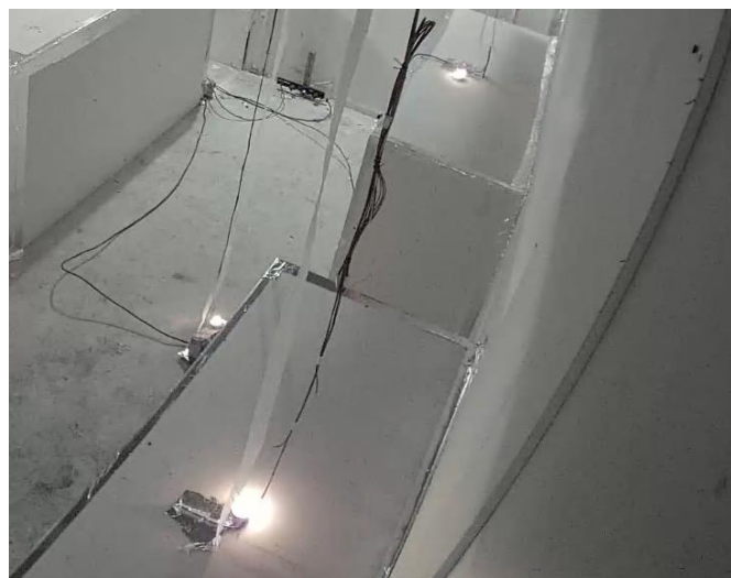
Candles Flaring up at 31 seconds after the beginning of the discharge due to increased refrigerant concentration.
