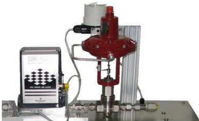
Figure 164 - Other\Mass Flow Control System
