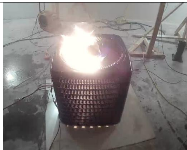
Video still showing ignition (62 s after release start)
