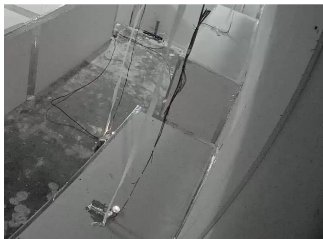
Candle at Locations C extinguished at 42 seconds after the beginning of the discharge. The blower motor had been operating for 10 seconds. The candle at location A extinguished 11 seconds later.
