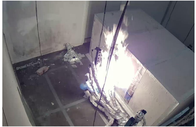
Ignition of the Refrigerant after Second Attempt
